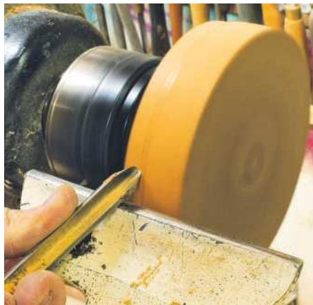
▲ Pic.5 True up the base with the bowl gouge. Keep the bevel pointing in the direction of the cut and keep the flute pointing at 10 o'clock to achieve the best finish
